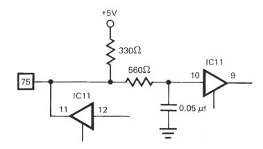
Provision of a 10  $\mu$ sec delay permits the memory board to turn off before the CPU terminates the current operation.
