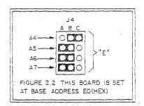
Secondly, the user should select the board I/O address. If the board is 8 bit addressed, then only jumper area J4 affects board address. The user may select address bits 4 through 7. See Figure 2.2.
