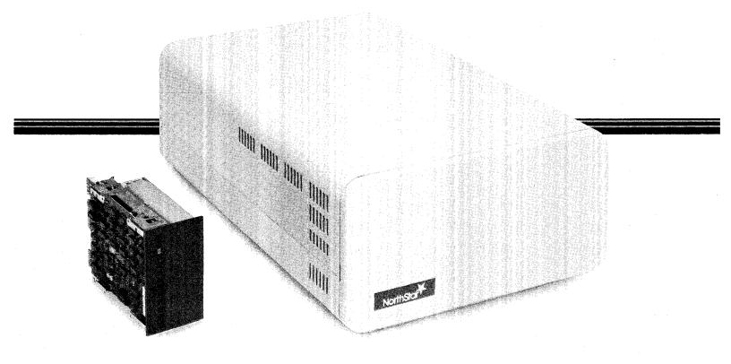
5Mb or 18Mb Winchester Technology/Hard Disk Subsystems for HORIZON® Computers. Drives May Be Added To A HORIZON Computer, And Are Supported By All North Star Software.
