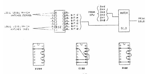
FIGURE 1P: PROM ADDRESS HEADER (LOCATION SE), WITH THREE EXAMPLES.
