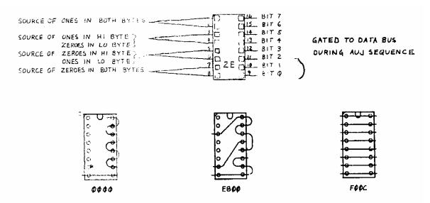
FIGURE 12: AUJ (POJ) ADDRESS HEADER (LOCATION 2E), WITH THREE EXAMPLES.
