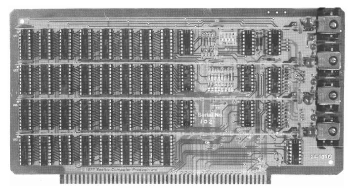
This board is fully compatible with the S-100 bus and should interface without difficulty to the MITS 8080, IMSAI, Poly 88, Sol 20, Cromemco, Alpha-Micro, and similar microprocessor systems. It was designed to operate without wait states with a Z-80A processor operating at 4 Mhz. when populated with the 250 nsec. memory chip. With the 450 nsec. chip, it will operate in 2 Mhz. systems without wait states. Its fully static design ensures "no clocking or interference problems" when used for DMA.
