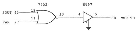
If you want to use the Tarbell Floppy Disk Interface with a Z-80 CPU board, you will need to either have read-only memory (ROM) somewhere else in your system, or to make the modifications listed below, to boot up properly. This is because most Z-80 CPU boards do not create the same kind of bus signals as the ALTAIR\* or IMSAI CPU boards.
