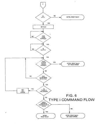
'NOTE: \*1. IF TEST - D. THERE IS NO 10MS DELAY. 2. IF TROF - 1 AND CLK - 1 MHz, THIS IS A 20MS DELAY.
