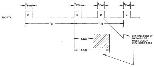
NOTE: INTERNAL DATA SEPARATION MAY WORK FOR SOME APPLICATIONS. HOWEVER, FOR APPLICATIONS REQUIRING HIGH DATE RECOVERY RELIABILITY, WDC RECOMMENDS EXTERNAL DATA SEPARATION BE USED.
