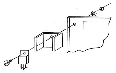
Turn board over and solder 3 leads to pads. Cut off any excess leads.
