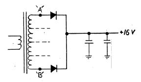
Connect the second end of the jumper from motherboard pin 64 to either point "A" or point "B" above. This is to the anode side of one of the diodes, signified as the end of the diode without the bands marked on it.
