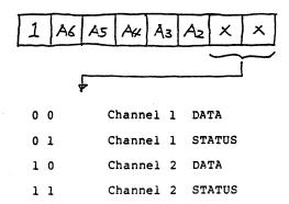
If the I/O addresses are set at the addresses COH to C3H then the board is usable with NBASIC. The switch settings corresponding to this setting are shown below.
